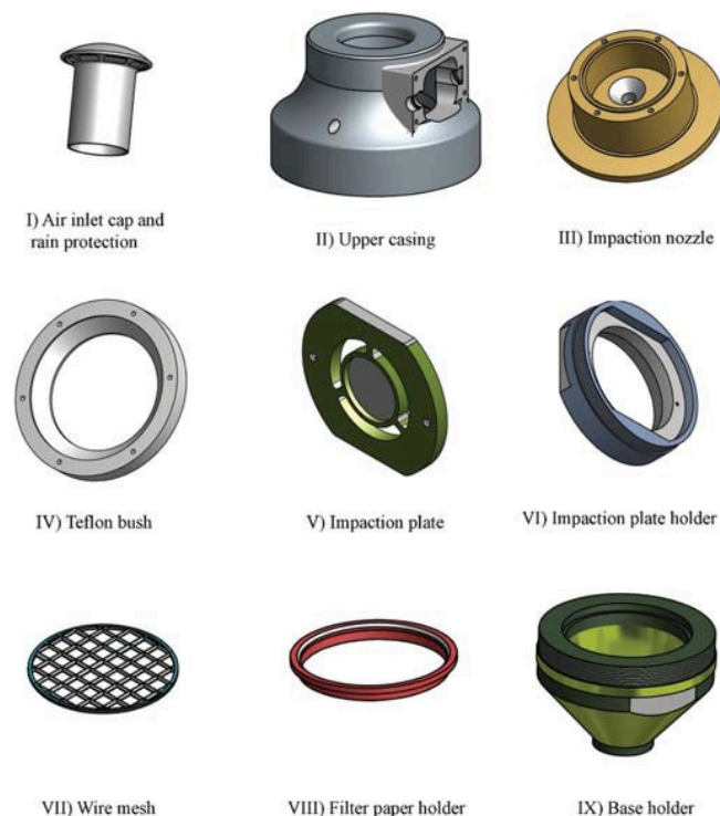
Figure 3b: Individual components of the novel inertial impactor
