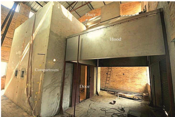
Fig.1b. View of Large-scale heat release calorimeter
