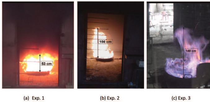
Fig. 5: Luminous flame height at time of 900 s
