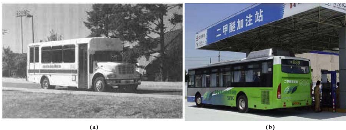
Fig. 3. (a) DME-Fueled Shuttle Bus, Pennsylvania (2002) and (b) DME-fueled bus and DME filling station in Shanghai, China (2009) [Fleisch et al. 2012]
